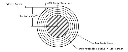
The winch torque capacity is 1950 in-lbs for the 1200 series gears.
