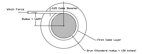
The winch torque capacity is 1950 in-lbs for the 1200 series gears.
